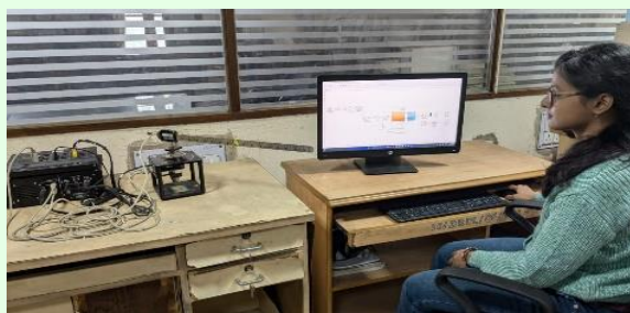
Implementation of a Data Driven Controller on Rotary Servo Flexible Link System interfaced with SIMULINK Real Time Workshop
